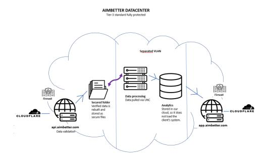
After the Performance metrics are received and validated by our API, the data is rebuilt and stored as **secured files**.
