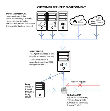
The Agent collects **WMI and System queries data** and sends to our API Cloudflare-secured address <u>api.aimbetter.com</u> via **SSL** ports through **secure Protocol TLS 1.2** after the Data **is encrypted** and compressed. The default outbound port is 443.
